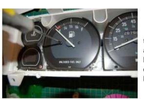
5. Choose your first gauge. You may find that the gauges are dusty... clean with a dry soft cloth and an air-duster. Remove the 2 screws (some may also have washers) and set these aside. We recommend one of the smaller gauges first, as the larger ones have an extra step and obstructions.
